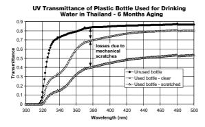
bottles. The figure on the left shows the transmittance losses due to mechanical scratches whereas the figure on the right illustrates the losses due to photoproducts. Smooth and careful cleaning is necessary to avoid mechanical scratches.
