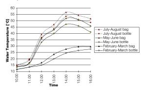
Wter temperature curves in bottles and bags. The average temperature difference is about 2-3 °C.
