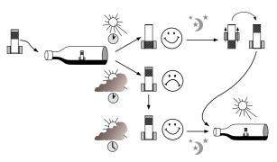
Use of the Temperature Sensor. After the paraffine has melted down, the screw is pulled up, making the sensor ready for use again.
