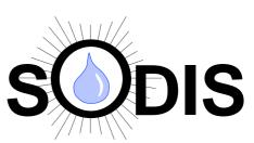
SODIS Logo for Turbidity Test. If one can read the letters, the turbidity is less than 30 NTU. If one can see the sun rays of the Logo, turbidity is less than 20 NTU.
