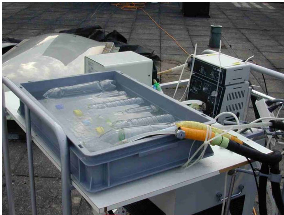
Figure 5: Detail of experimental set-up for sunlight exposure at 60°C.
