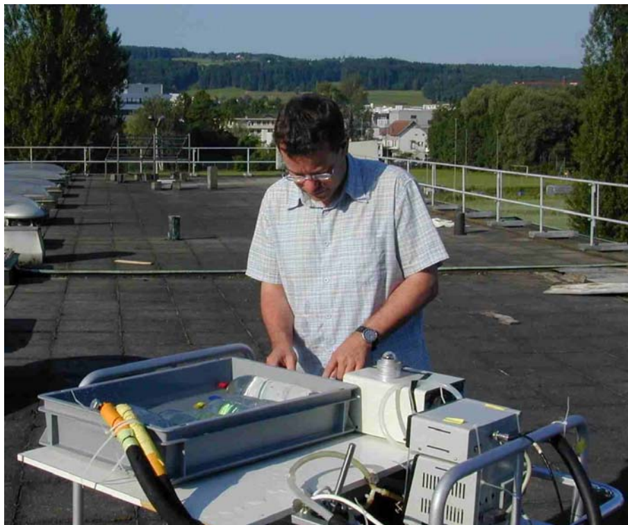
Figure 3: Experimental set-up for sunlight exposure at 60°C.
